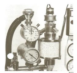
Fig. 2 Minute Volumeter 3000 in circle system of anaesthetic machine
