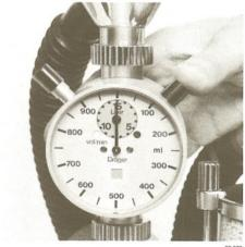
Fig. 4 Release of indicator hand for tidal volume
