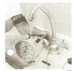
Fig. 8 Flushing out Volumeter
