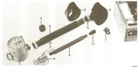
Fig. 5 Dräger Minute Volumeter 3000 with special equipment kit
