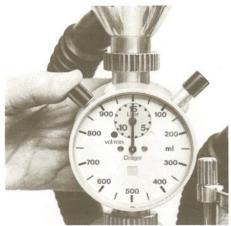
Fig. 3 Release of indicator hand for minute volume
